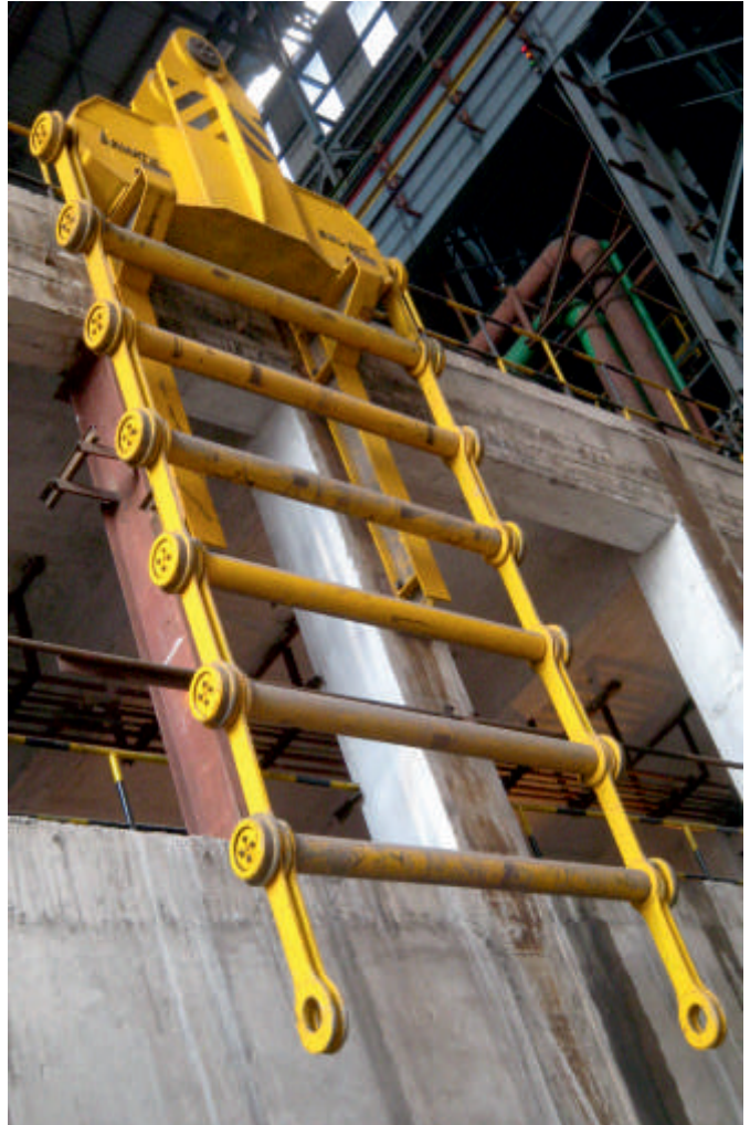
60MT Link Chain - Tundish Beam
